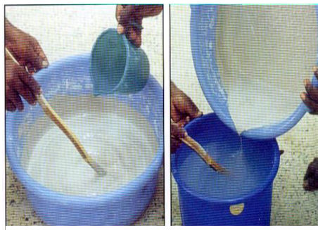
Preparation of Bleaching Powder paste & mixing the paste with water
